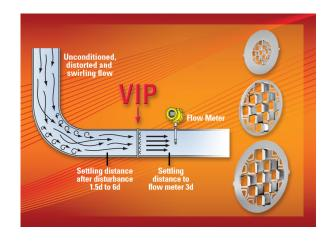
greatly reduces the pressure drop compared to alternative technologies such as tube bundles, screens and perforated plates. Minimizing pressure drop is a significant design consideration in flow conditioning for process engineers to minimize plant energy consumption and energy costs.
